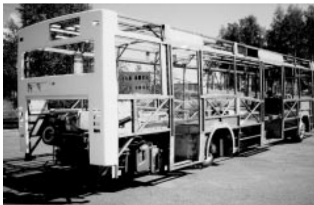
Fig. 1 Structure of the stainless steel bus frame
